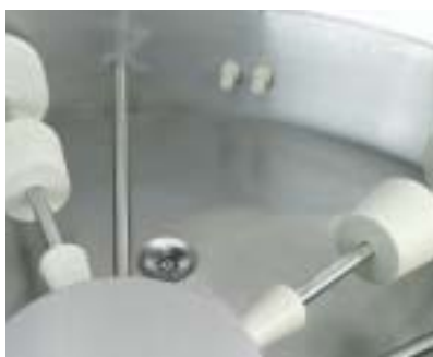
Drain in the bottom of the basin.
